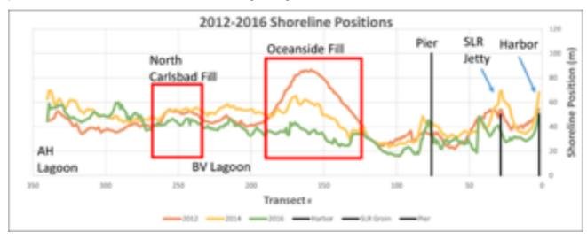
Figure 8 2012-2016 Measured Shoreline Positions and RSBP II Fill Locations
