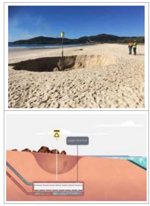
Figure 11-2. Mobile Sand Bypass Option – Sandshifter Detail (Swash, 2021)
