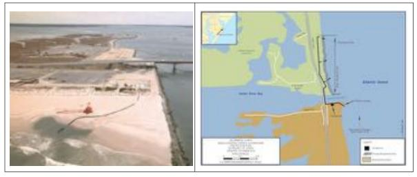
Figure 11-3. Mobile Sand Bypass Option – Indian River Inlet, Delaware (USACE, 2021)
