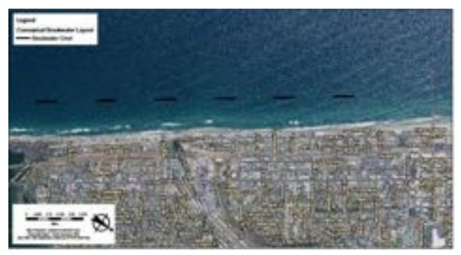
**Figure 12 Artificial Reef Full Layout Position**
