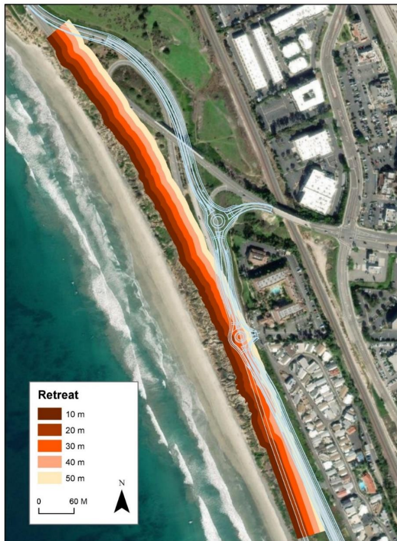
Figure 18. Map of the forecast area showing proposed road alignment and zones of cliff retreat relative to the 2020 cliff top position.
