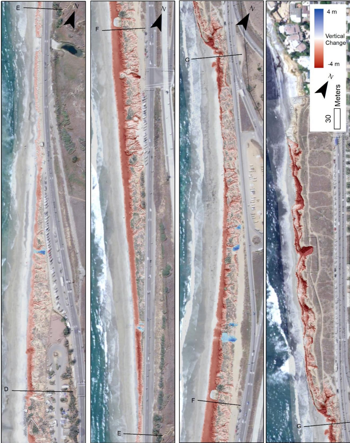
Figure 12. Vertical change maps of the north portion of the study showing erosion (red) and deposition (blue) between 1998 and 2020. Colors saturate at +/- 4 m. From left to right, the panels go northward. Matchlines between panels and Figure 11 are indicated.
