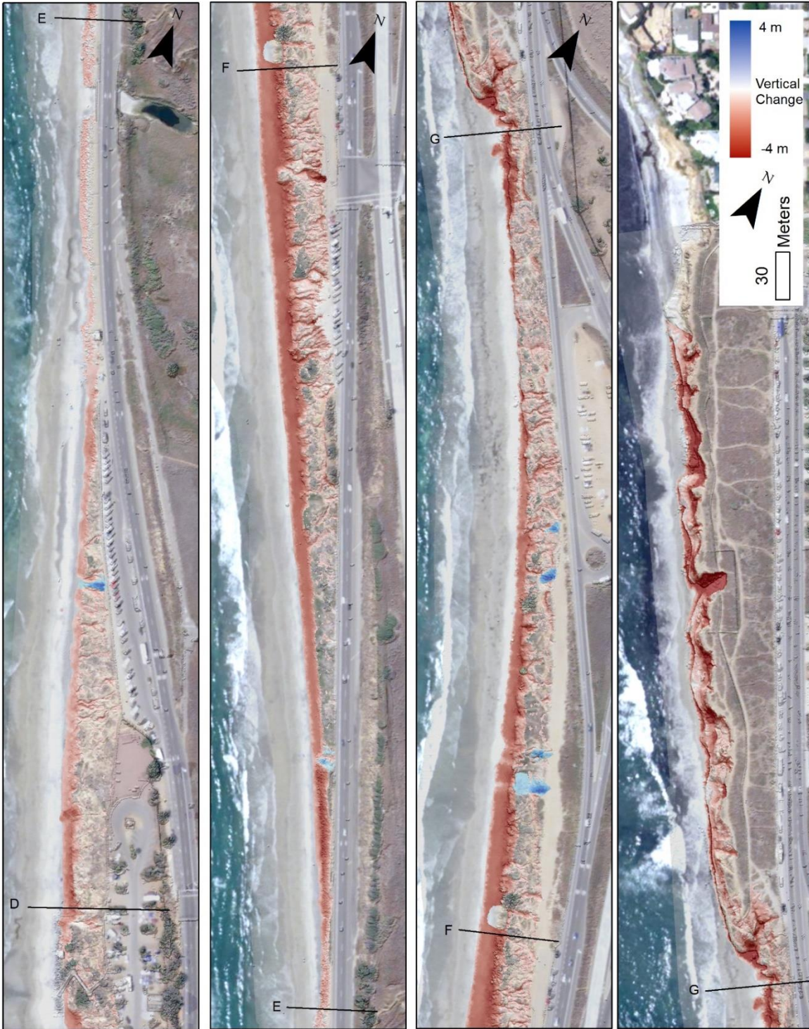
Figure 12. Vertical change maps of the north portion of the study showing erosion (red) and deposition (blue) between 1998 and 2020. Colors saturate at \pm 4 m. From left to right, the panels go northward. Matchlines between panels and Figure 11 are indicated.
