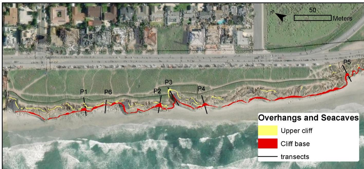
Figure 8. Areas with over-vertical topography in the upper and lower cliff obtained from a Sept. 17, 2020 LiDAR survey combined from drone- and truck-based mobile LiDAR systems. Labeled cross shore transects are shown in Figure 9.
