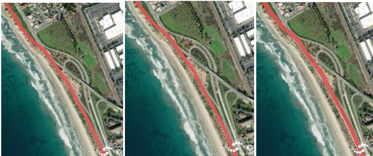
Figure 6. Example CoSMoS 3.0 Phase 2 projected cliff retreat for 2.5 ft (0.75 m), 3.3 ft (1 m), and 6.6 ft (2.0 m) of sea level rise within the study area (source: Our Coast Our Future online viewer). Red is the zone of cliff retreat.
